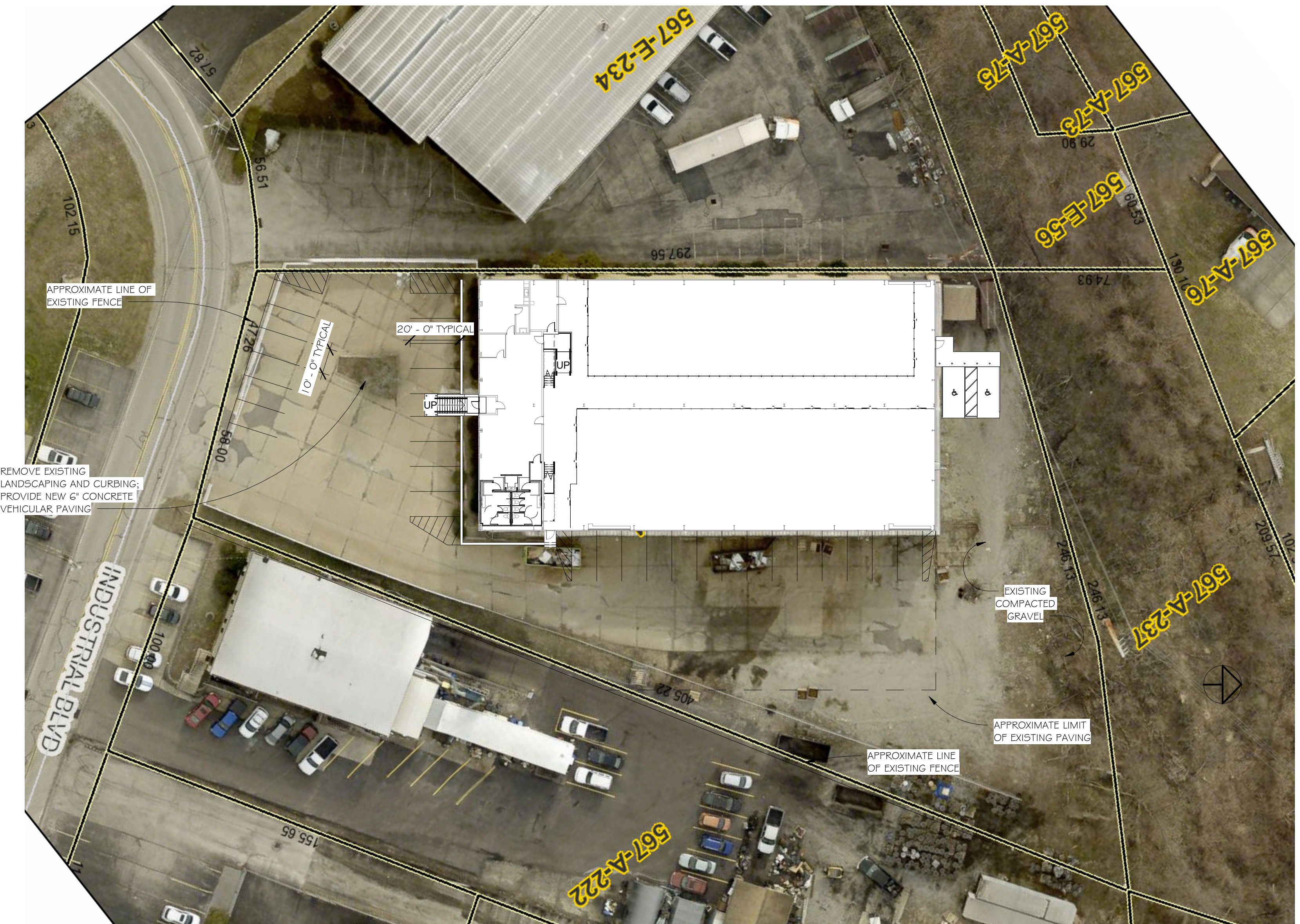
1 Site plan A003 1" = 30'-0" NOTE: BACKGROUND IMAGE SCALE IS APPROXIMATE. PROPOSED PARKING TOTAL: 30 SPACES ACCESSIBLE: 2 SPACES
